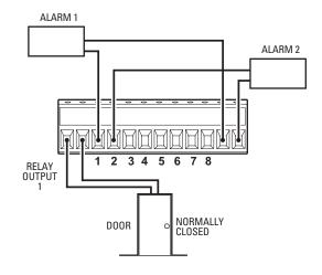
Figure 9. Alarm and Relay Wiring
